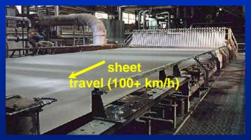
Several hundred sensors and actuators, millisecond operation, controlling paper thickness to within microns!
