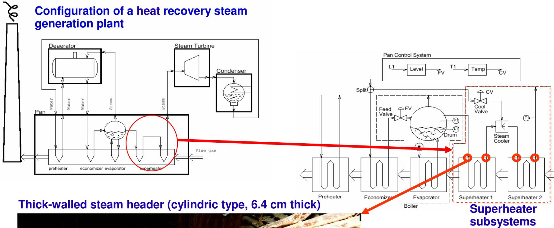
**Thick-walled steam header (cylindric type, 6.4 cm thick)**
