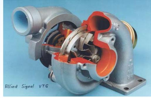
Variable geometry turbocharger with pneum/electr. actuator
