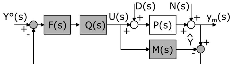
Figure 19: IMC block diagram.
