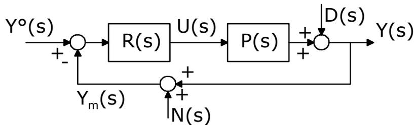
Figure 2: generic linear 1-d.o.f. (PID) feedback control scheme.
