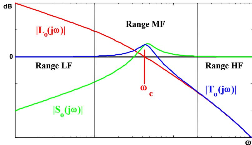
Figure 9: important ranges in frequency domain design.
