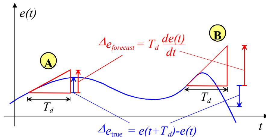
Figure 3: explanation of the role of the D action.
