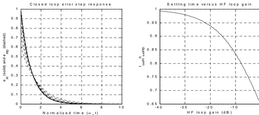
Figure 25: PI versus PID tuning with ISE minimisation.
