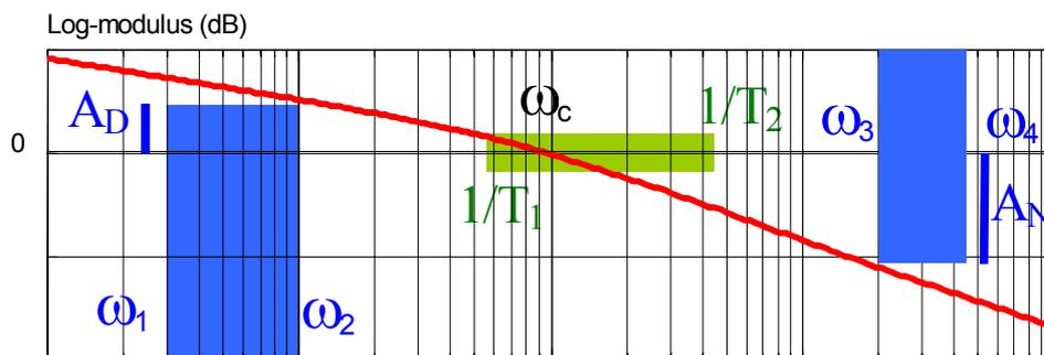
Figure 7: the Bode magnitude diagram as assessment tool.
