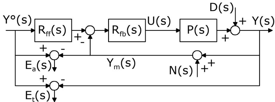
Figure 8: generic feedback control scheme highlighting the true and apparent errors.
