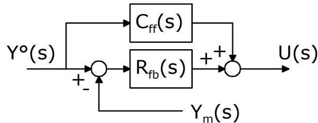
Figure 12: set point weighting viewed as feedforward compensation.
