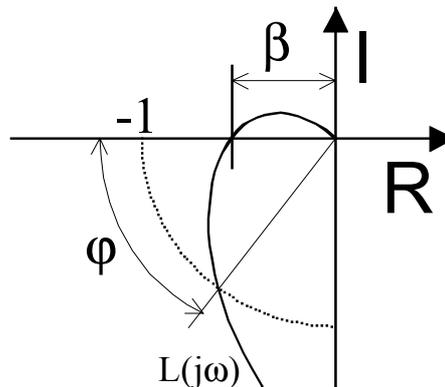
Figure 5: gain and phase margins as seen on the Nyquist diagram.
