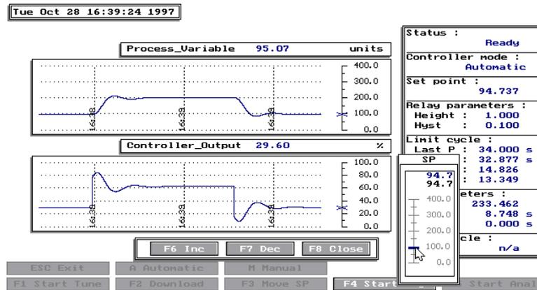
Figure 31: CAD software screen dump showing evaluation of PI controller
