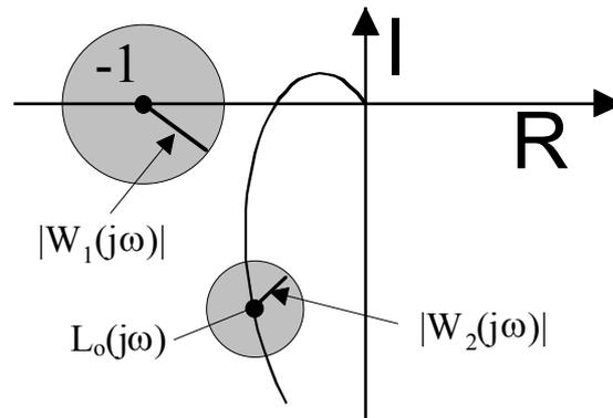
Figure 10: assessing robust performance on the basis of  $S_o(j\omega)$  and  $T_o(j\omega)$ .
