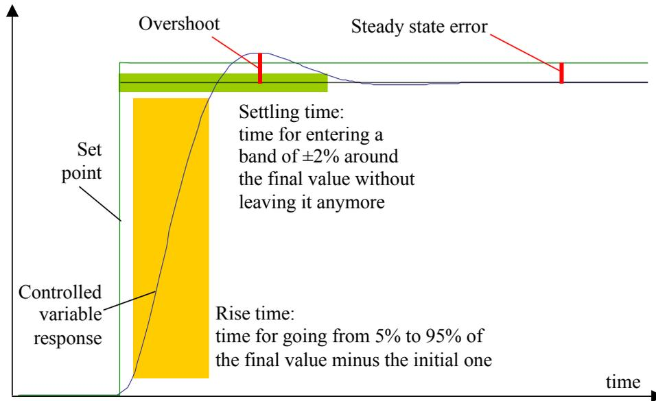
Figure 4: typical requirements for the closed loop step response in the time domain.
