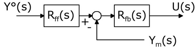
Figure 11: a PID regulator with 2 degrees of freedom.
