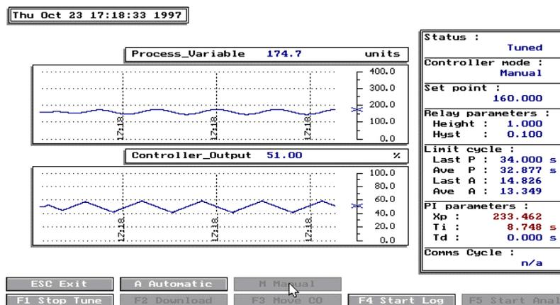
Figure 30: CAD software screen dump showing Autotuning in process
