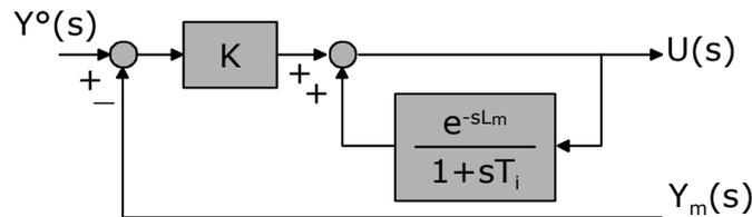
Figure 14: the basic scheme of the predictive PI (pPI).
