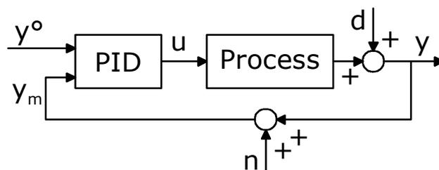
Figure 1: generic PID control scheme.
