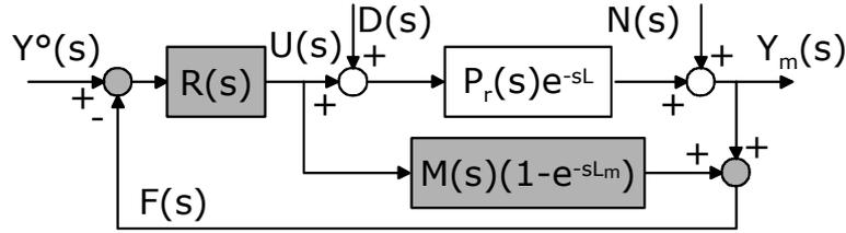
Figure 13: the basic scheme of the Smith predictor.
