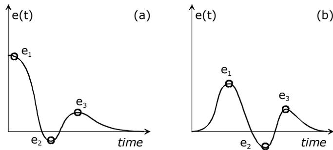
Figure 26: examples of error transients for (a) a set point change and (b) a load disturbance.
