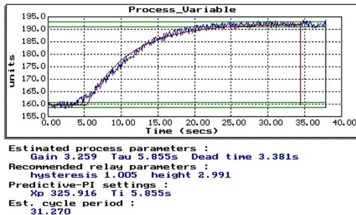
Figure 29: typical process analysis result
