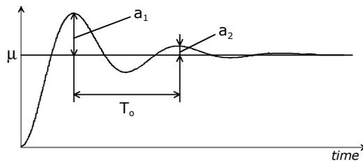
Figure 17: estimating second order oscillatory models.
