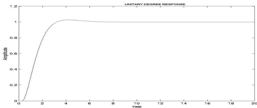
Figure 34: a step response obtained with MOGA PID autotuner
