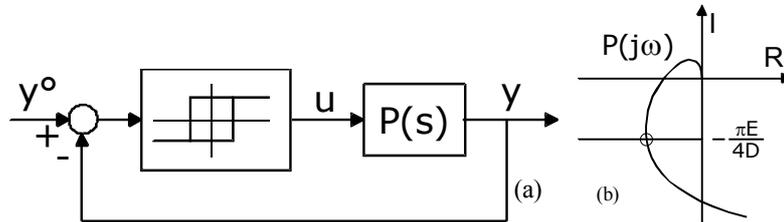
Figure 18: relay feedback (a) and oscillation characteristics (b).
