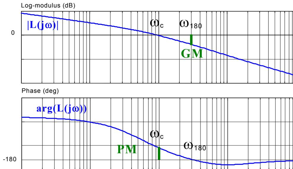
Figure 6: gain and phase margins as seen on the Bode diagrams.
