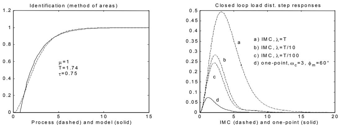
Figure 22: different tuning operations on the same process.
