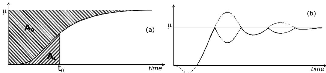
Figure 16: the method of areas (a) and the response to be used (b).
