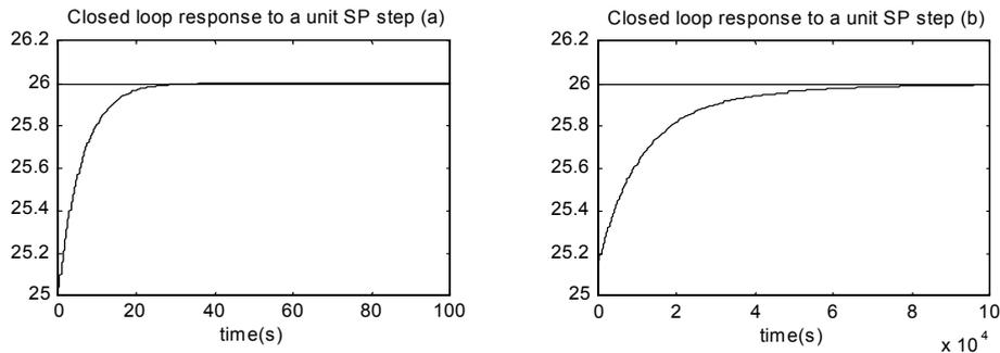
Figure 24: closed loop responses with and without detrending.
